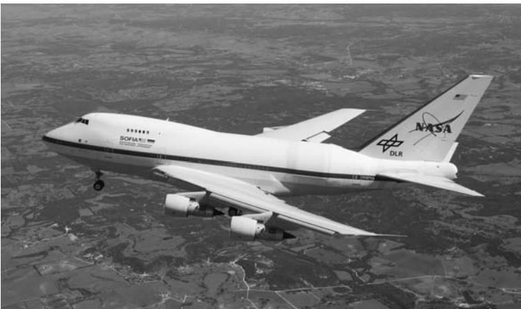
Fig. 7.12 The SOFIA facility will fly at about 12 km altitude, above most of the water in the earth’s atmosphere. This will allow measurements in the sub-mm and far infrared range. The modified 747SP airplane contains a 2.5 m optical telescope. This is a joint project of NASA and the German Space Agency, DLR. The first test flights are now taking place
