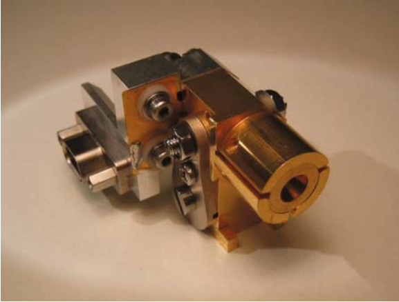
Fig. 5.12 [An ALMA Band 9 SIS mixer] A photo of the feed horn on the right, and the SIS mixer holder on the left. This was built at the Space Research Organization of the Netherlands (SRON). This receiver covers the frequency range 610–720 GHz. This is a tunerless double sideband mixer. This is typical for the sub-mm SIS mixers used in the ALMA instrument
