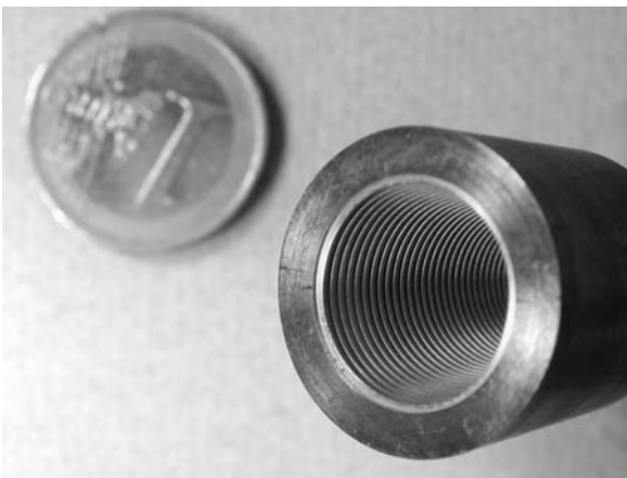
Fig. 7.5 A corrugated waveguide hybrid mode feed for \lambda 2 mm for the IRAM Plateau de Bure interferometer (courtesy of B. Lazareff)
