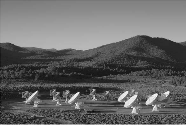
Fig. 9.8 The Combined Array for Research in Millimeter-wave Astronomy (CARMA) is located in northern California, at an elevation of 2.2 km. CARMA is the merger of the Owens Valley Radio Observatory (OVRO) millimeter array (consisting of six 10-m dishes) and the Berkeley-Illinois-Maryland Association (BIMA) array (consisting of nine 6-m dishes). Funding for CARMA is provided by the U. S. National Science Foundation and the consortium universities (photo courtesy of J. Miller and D. Bock)
