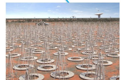
SKA1_Low 50 – 350 MHz 131,000 aperture array dipole 512 stations of 256 antennas
